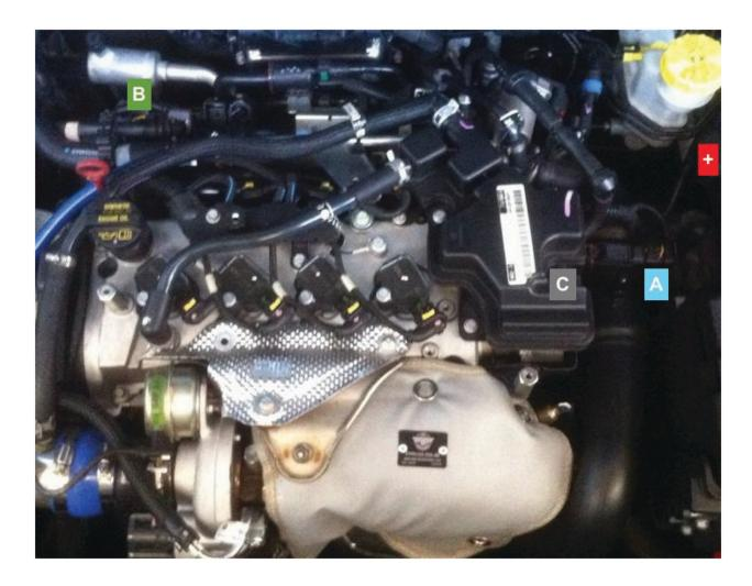
The image above shows the location of the sensors the MAXPower PRO taps into.
